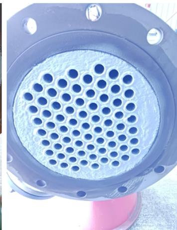
Tube sheet preparation complete grit blasted and cleaned
