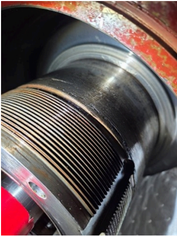
Damage on shaft caused by a spun bearing in service
