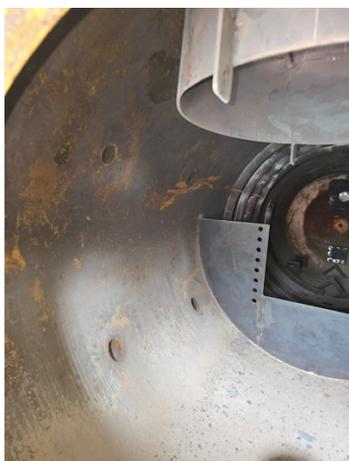
The Test separator suffered severe erosion-corrosion, compromising equipment integrity and safety.
