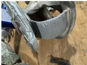
Belzona 1111 Formed to Fill Missing Area and then wrapped with Reinforcement Cloth and More Belzona 1111
