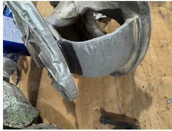
Belzona 1111 Formed to Fill Missing Area and then wrapped with Reinforcement Cloth and More Belzona 1111
