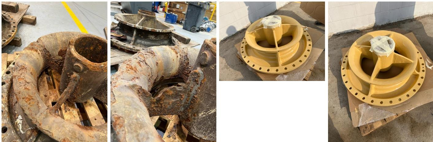
The suction bells exhibit severe corrosion and erosion as a result of prolonged exposure to saltwater.
