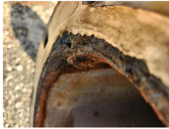
Close-up of the damaged flange face on the stainless-steel sand filter spool.
