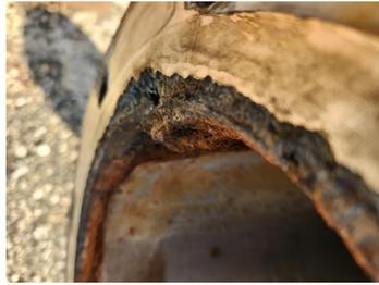
Close-up of the damaged flange face on the stainless-steel sand filter spool.
