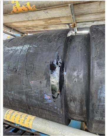
Large tears and gouges reduced the efficacy of the Fender and caused ropes to become caught
