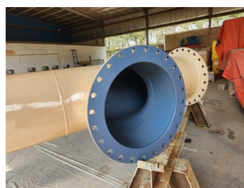
Application of Belzona 1321 (Ceramic S-Metal), an erosion-corrosion resistant lining, applied internally.
