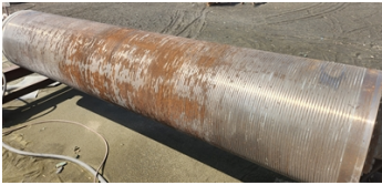
A dryer roller suffered corrosion & erosion attack
