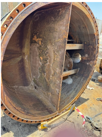
A heat exchanger channel head in a petrochemical plant had suffered significant corrosion-erosion, resulting in wall-thickness loss.
