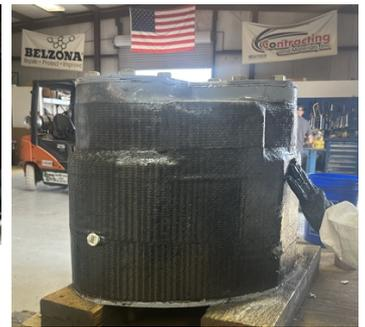
FINAL PHOTO SHOWS HOW WE WRAPPED THE ENTIRE VALVE BODY USING BELZONA 1984 AND CARBON FIBER SUPER WRAP. WE APPLIED 6 WRAPS TO THIS APPLICATION FOLLOWED BY BELZONA 9382 RELEASE FILM TO COMPRESS THE WRAPS AND 1984.
