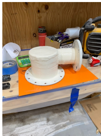
External repair completed on the top nozzle piece
