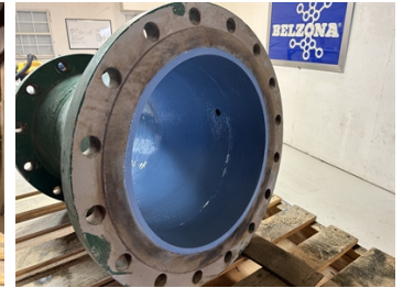
Completed photo of spool piece with two coats of Belzona 1321
