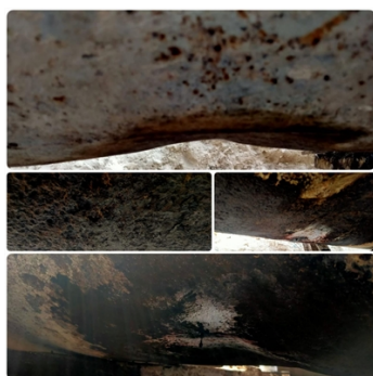
Pipeline damage caused by severe external corrosion
