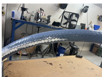
Applying 5821 with Cabosil to fill in as a grout and add some wear resistance.
