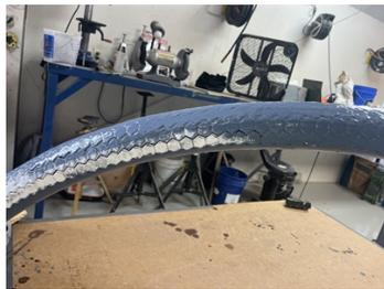
Applying 5821 with Cabosil to fill in as a grout and add some wear resistance.
