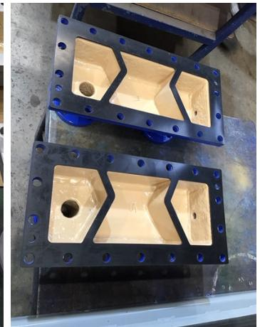
This section shows the original condition of the end caps prior to refurbishment.
