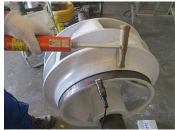
After the second coat of Belzona 1331 was fully cured, it was inspected for holidays/pinholes with a PCWI low voltage tester and successfully passed.
