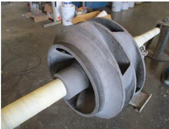
Carbon steel surface prepared by grit blasting with steel grit to give a minimum depth of 75 microns and surface cleanliness by Swedish standard Sa 2.5
