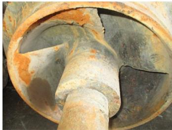
Pump impeller showing damage caused by erosion and corrosion
