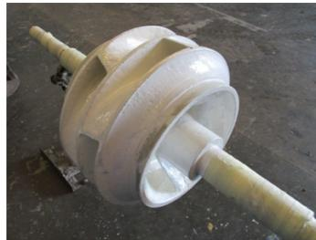
The first coat of Belzona 1331
