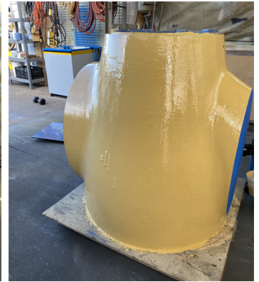
Belzona 5821 Second Coat
