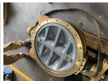
Two coats of Belzona 1321 (Ceramic S-Metal) were applied to provide enhanced protection.
