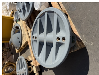
Belzona 1311 (Ceramic R-Metal) was used to rebuild the damaged areas.
