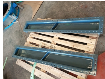
The covers were rebuilt using Belzona 1111 (Super Metal) and coated with Belzona 1321 (Ceramic S-Metal).
