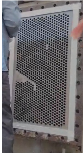
Tube sheets after abrasive blasting to SSPC-SP10 / ISO 8501-1 Sa 2.5 cleanliness standards.
