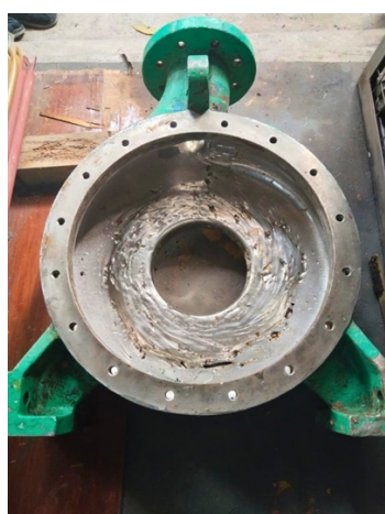
Severe abrasive wear and leakage
