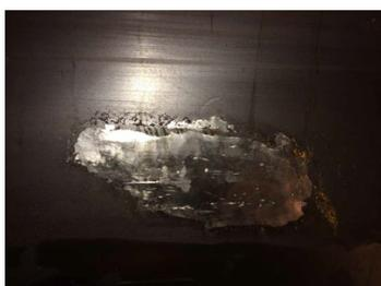
Damage to the impeller
