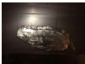
Damage to the impeller
