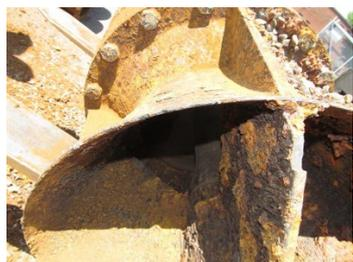
Corroded suction bell needed repair
