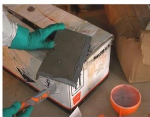
Applying Belzona Compound to Metal Plates
