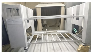
Construction after blasting
