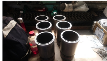
Inserts and engine cylinders were chemical wash up
