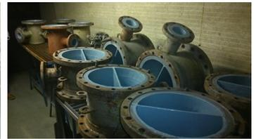
The coated equipment was placed in the oven. The temperature was raised so that the coating was heated to a minimum 50°C for 1 hour.
