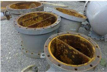
Erosion and Corrosion to the exchanger parts required repairing.
