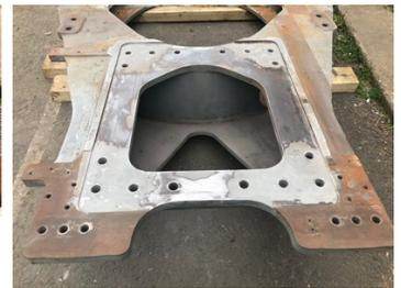
The Belzona 1111 machined flat with the surrounding metal
