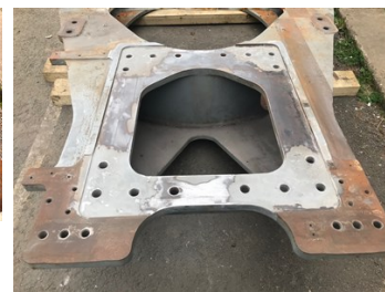
The Belzona 1111 machined flat with the surrounding metal
