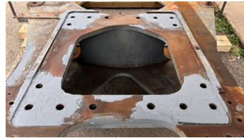
Belzona 1111 built up proud of casing
