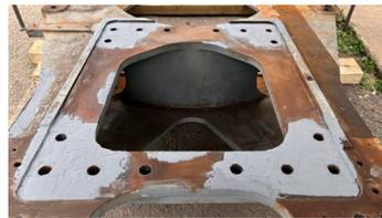
Belzona 1111 built up proud of casing
