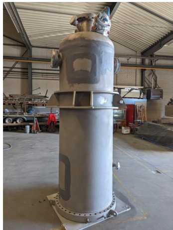
Plate bonding applied
