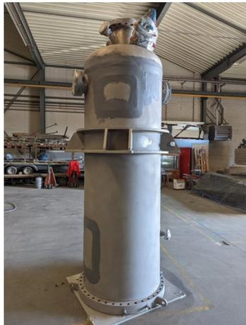
Plate bonding applied
