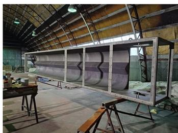
Screw troughs coated with Belzona 1812 to protect the steel substrate.
