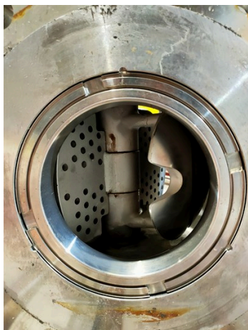
Valve showing internal parts
