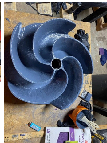
Impeller rebuilt with expanded metal, Belzona 1111 Supermetal, and coated with Belzona 1321 S-Metal.
