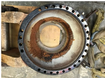
Before / Damage on the Nozzle head
