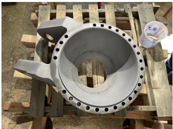
After abrasive blasting to SSPC SP-10/3 mil profile Surface Preparation
