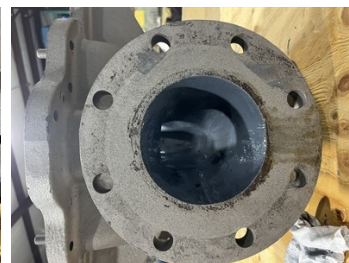
Second view of Belzona 1321's second coat.
