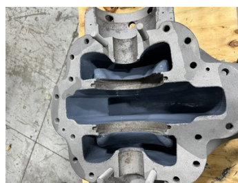
Second Coat of Belzona 1321 (blue).
