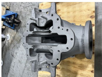
Pump after being sandblasted/prepared.
