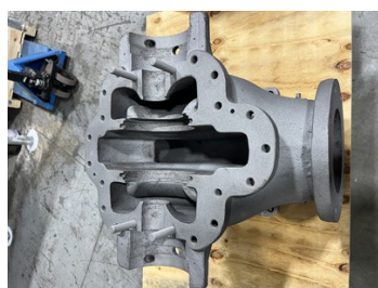
Pump after being sandblasted/prepared.
