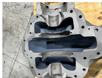
Second Coat of Belzona 1321 (blue).
