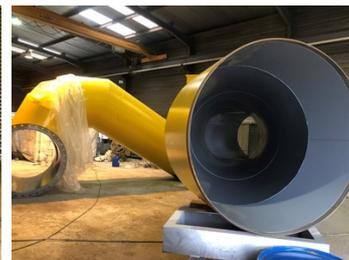
Finished internal & external lining application using Belzona 5811.
