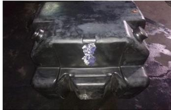
Cracked and leaking fuel tank
