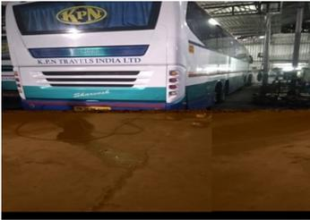
Bus with fuel tank leakage problems
