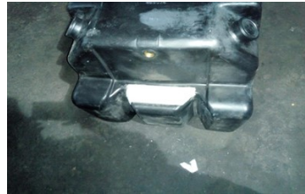
Fuel tank that has been repaired and is no longer leaking
