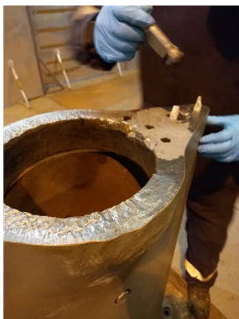
Surface preparation carried out & Belzona 1111 applied
