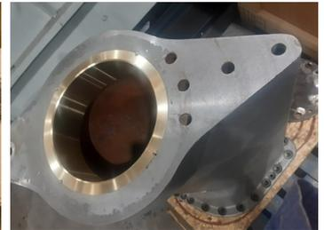
Surface preparation carried out & Belzona 1111 applied
