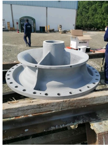
After repair with Belzona 1111
