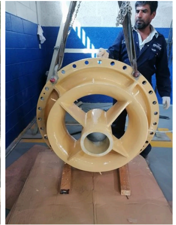
After coating with Belzona 5821
