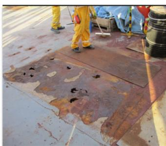
Holes in the surface plate of the deck due to severe corrosion
