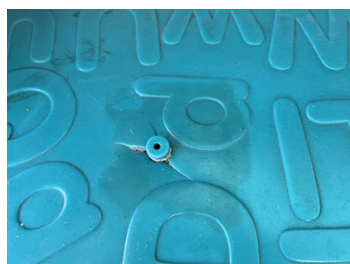
Blow holes with cracks formed around it
