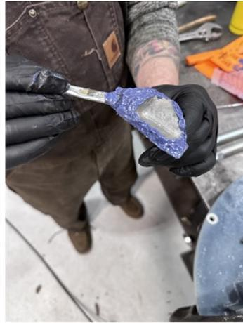
Applying 7311 to Broken Piece
