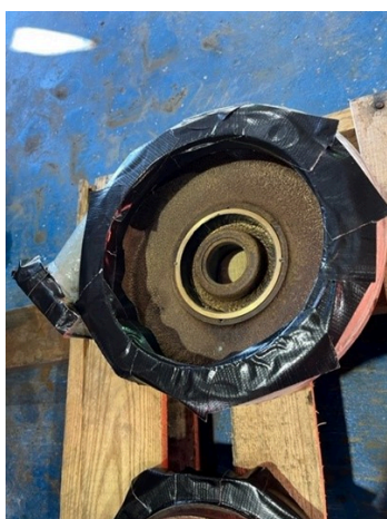
Casing showing sings of extreme erosion from years of sandy water service.
