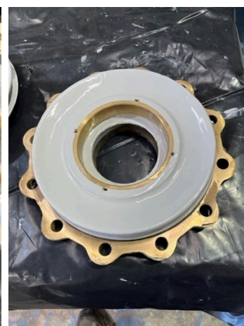
Backing plate feeling young again after being rebuilt and coated.
