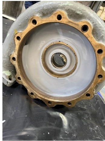
Freshly rebuilt and coated casing ready for more years of service.
