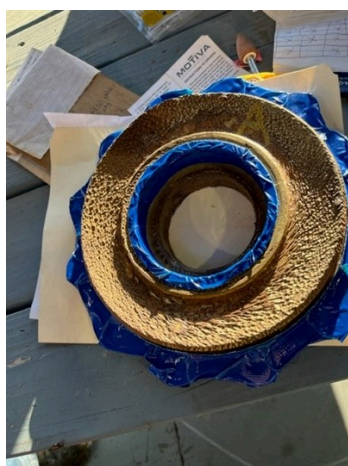
Backing Plate showing sings of extreme erosion from years of sandy water service.
