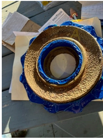
Backing Plate showing signs of extreme erosion from years of sandy water service.
