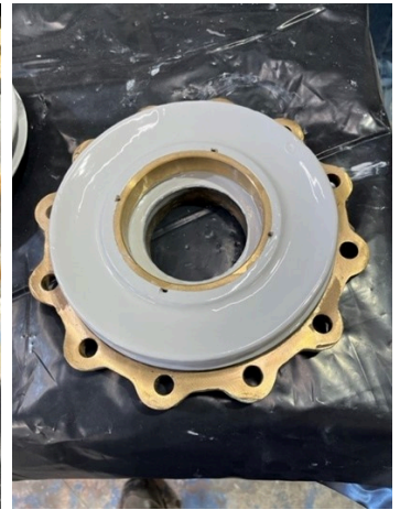
Backing plate feeling young again after being rebuilt and coated.
