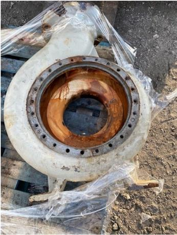
Casing before coating showing wear from service
