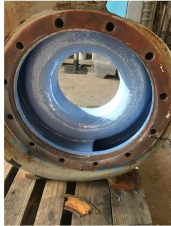
Freshly rebuilt and coated pump casing
