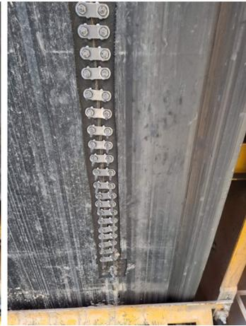
Belt fasteners installed
