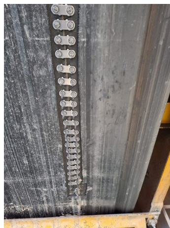
First layer of the belt peeled off in order to install belt fasteners properly
