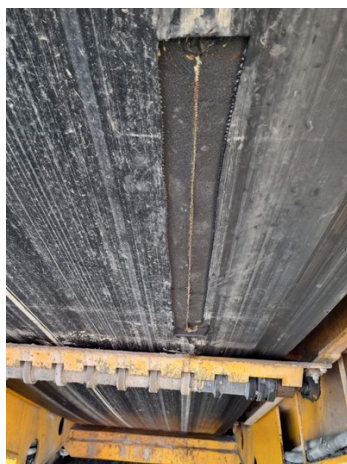
First layer of the belt peeled off in order to install belt fasteners properly
