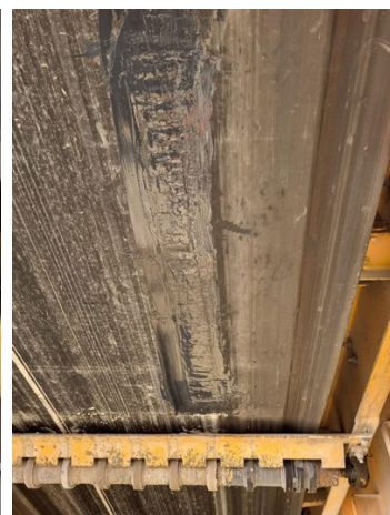
Belt fasteners protected with Belzona 2311
