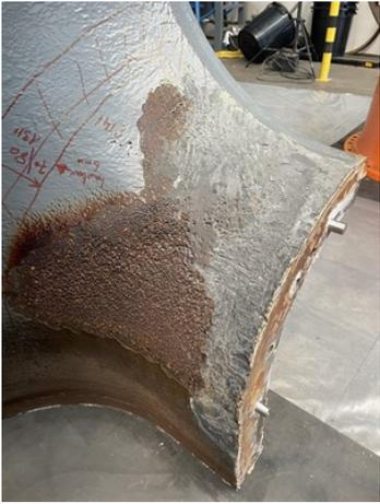
Damage caused by erosion-cavitation leading to a substrate loss greater than 5mm.
