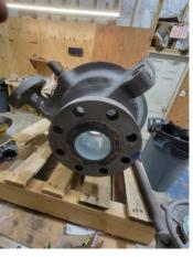
Pump internals after it was abrasive blasted. Two small holes shown.
