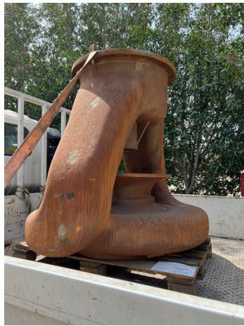
Before application: external corrosion
