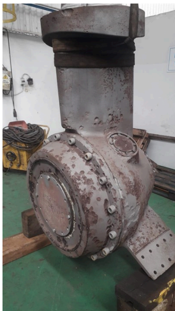
Before Application (showing the cavitation damaged areas)
