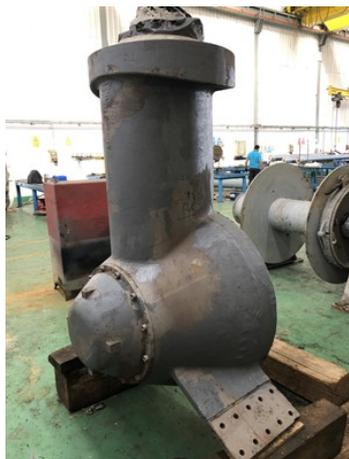
Belzona 1311 Applied for Repair
