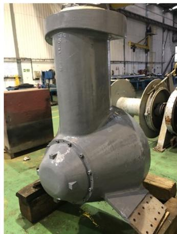
Belzona 1321 First Layer Coating Applied
