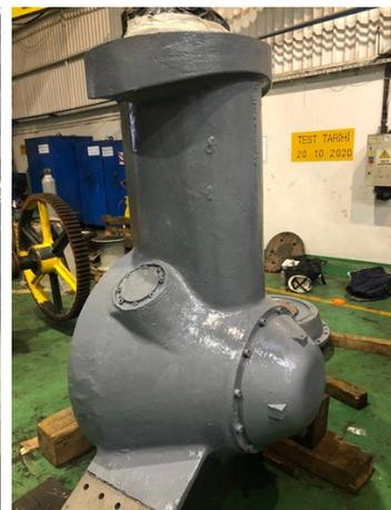
Belzona 1321 Second Layer Coating Applied
