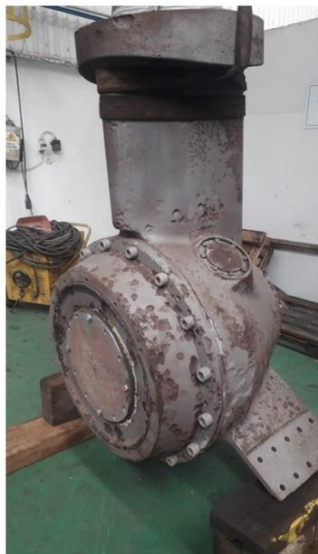
Before Application (showing the cavitation damaged areas)
