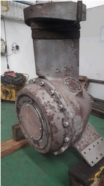
Before Application (showing the cavitation damaged areas)
