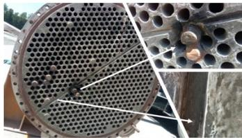
Eroded tubesheet and damaged division bar slot
